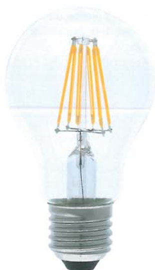
LCC-Standardlampe A60, 980 lm 2700K klar, 230 VAC 7 W E27, äquivalent 75-W-Glühlampe
