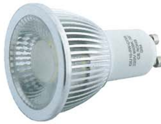
LCC-Spotlampe GU10, 430 lm 3000K 38° dimmbar, 230 VAC 5 W GU10
